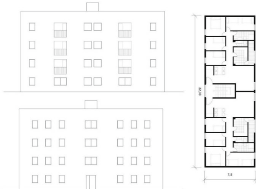
Fig. 3.5 Planimetry of the simulated building. From top to bottom: front views (north and south) and standard. Source Authors' own with data extracted from. "Typological analysis of linear social housing blocks: Spain 1950–1983. The case of Western Andalusia", Guajardo, A. (2017)
