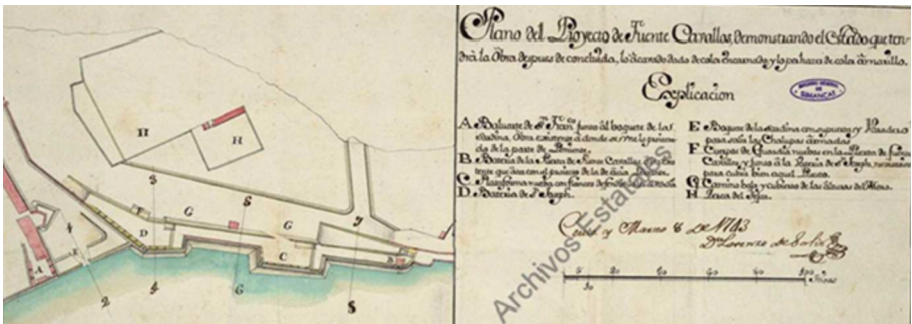
Fig. 6. Plan of the Project of Fuente Caballos, showing the condition that will have the work once concluded, the finished work in red and the work in progress in yellow - Lorenzo de Solís - 1743 - General Archives of Simancas - MPD, 19, 180 [9]
