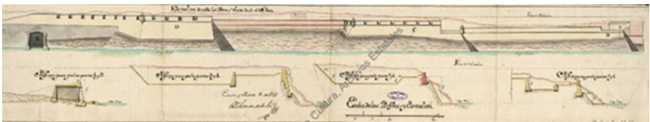
Fig. 7. Elevation of the work seen from the sea; Profile passing through point 1 and 2; Profile passing through point 5 and 6; Profile passing through point 7 and 8 - Lorenzo de Solís - 1743 - General Archives of Simancas - MPD, 12, 057 [9]
