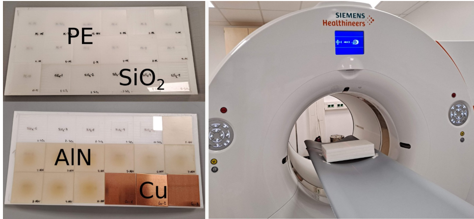
FIGURE 3.24: (Left) Positioning of the irradiated foils between the polyethylene thick layers. (Right) PET measurement of the activity of the irradiated foils embedded in the PE matrix at WPE.
