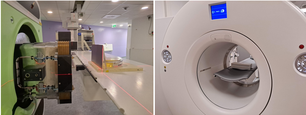
FIGURE 3.12: (Left) Irradiation of two graphite sheets. (Right) PET/CT measurement of the activated sheets inside the PE converter.
