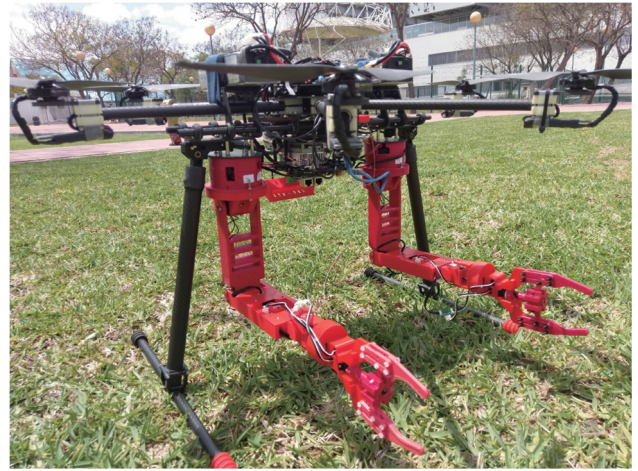
Fig. 1. A photograph of the arms built in the multirotor.
