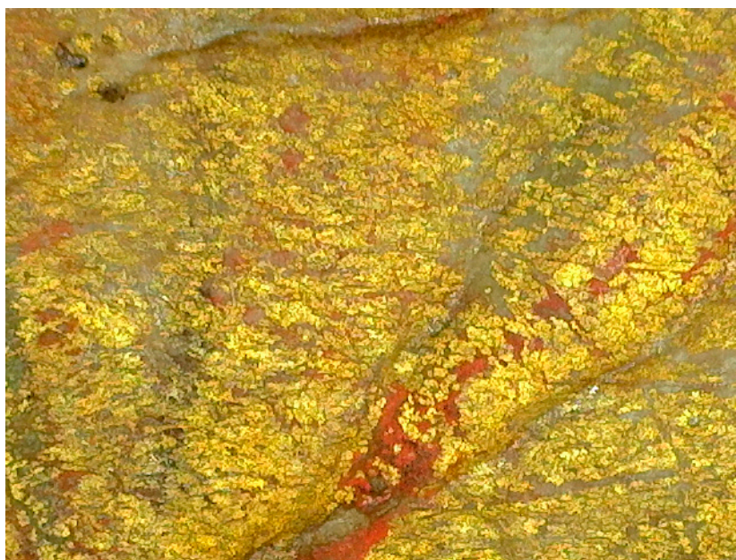
Figure 9. Gilded wind rose observed under digital Dino microscope. Gold foil was placed on a transparent mixture (reproduced with permission from the AGI).
