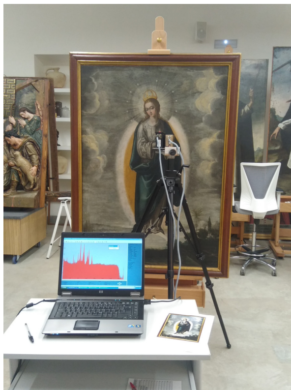
Figure 2. XRF in situ analysis of La Inmaculada .
