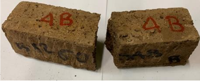
Figure 6 - failure mode of control sample (ID 0)
