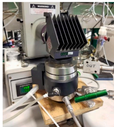
Fig. 1. Photocatalytic gas-phase flow-reactor used for thermo-photocatalytic runs.
