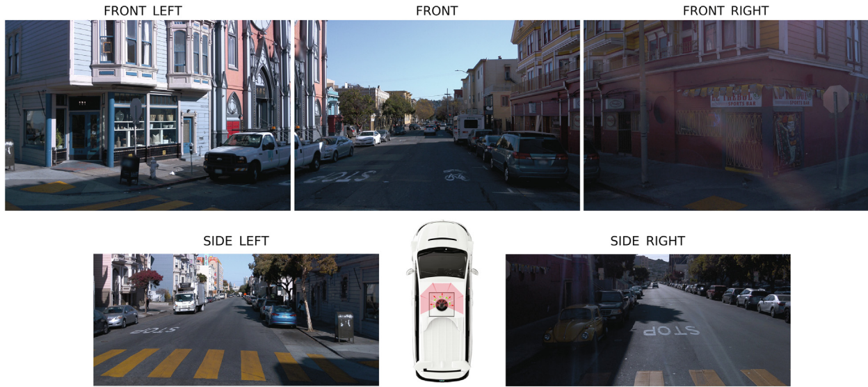
Fig. 1. Images from a single frame obtained by the five cameras of Waymo’s vehicle.
