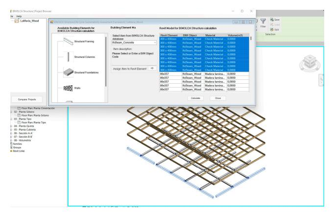
Figure 5. BIM3LCA. Null Element Material Volume Detection.
