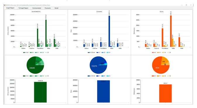
Figure 10. Results for Design option 1 (timber and reinforced concrete).
