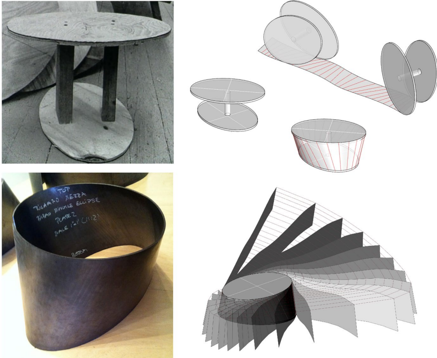
Fig. 6 Top left Rotary mechanism by Richard Serra. Image retrieved from the video Charlie Rose Conversation (2001), Time 33:32, reproduced by permission; Top right Calculating the developable surface on a plane with the rotary mechanism. Source: author; Bottom left Torqued Ellipse in Brancusi-Serra Exhibition at the Guggenheim Museum Bilbao between 2011 and 2012 . Photo: authors; Bottom right Movement of the sheet as it is unrolled, going from its flat to spatial form. Images: authors
