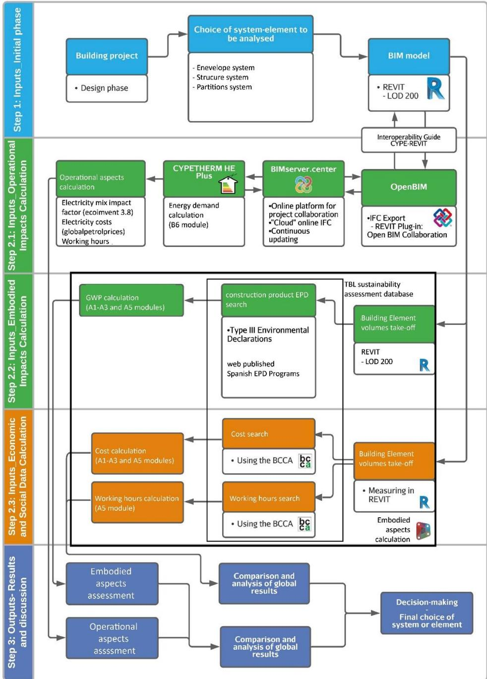
**Figure 1.** Schematic of the workflow and information requirements.
