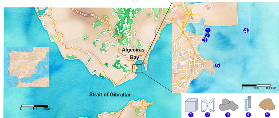
Fig. 1 Study area with 5 substrates (1 = Cubes, 2 = Acropods, 3 = Rip-Raps, 4 = Seawall, 5 = Natural)
