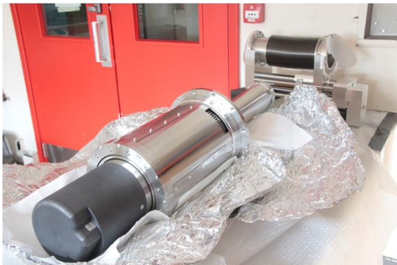
FIG. 6. Picture of the assembled MAST-U FILD.
