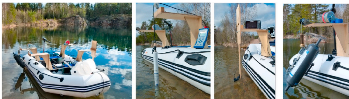
Fig. 2. Different probes and sampling systems used during this project. From left to right: the fully-equipped boat, Hydrolab M5 multiparametric water probe, Helix 5SI echo sounder and Niskin bottle.
