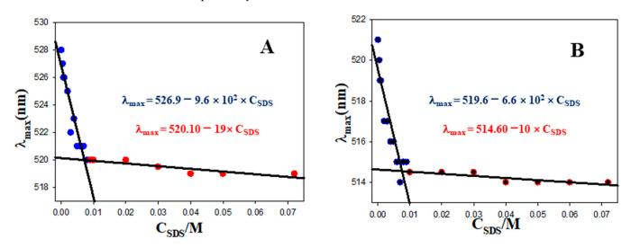
**Figure 2.** CMC determination for SDS surfactant following changes in maximum SPR wavelength. (**A**) Au@16-3-16/SDS system. (**B**) Au@16-6-16/SDS system.
