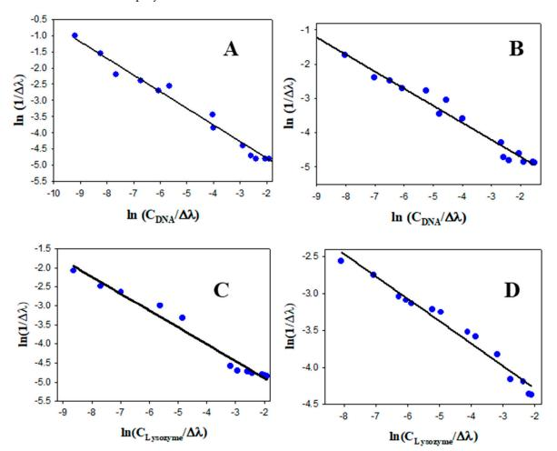
Figure 9. Colorimetric response patterns obtained with colorimetric sensors in water, showing the linear relationship between  $1/\Delta\lambda_2$  logarithms and the logarithms of the quotient between biopolymer concentration and  $\Delta\lambda_2$ . (A) Au@16-3-16/SDS/DNA system. (B) Au@16-6-16/SDS/DNA system. (C) Au@16-3-16/SDS/Lysozyme system. (D) Au@16-6-16/SDS/Lysozyme system.
