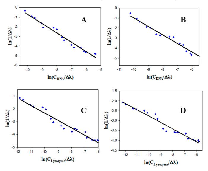
**Figure 10.** Colorimetric response patterns obtained with colorimetric sensors in horse serum media, showing the linear relationship between  $1/\Delta\lambda_2$  logarithms and the logarithms of the quotient between biopolymer concentration and  $\Delta\lambda_2$ . (A) Au@16-3-16/SDS/DNA system. (B) Au@16-6-16/SDS/DNA system. (C) Au@16-3-16/SDS/Lysozyme system. (D) Au@16-6-16/SDS/Lysozyme system.
