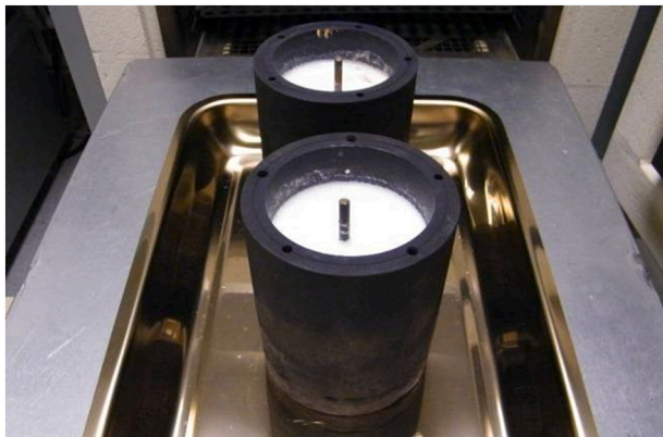
Fig. 2. Crucibles containing molten nitrate salt and corrosion coupons.
