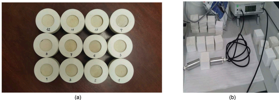
Figure 4. a) Containers with specimens for water vapour permeability test, b) Ultrasonic pulse velocity measurement.
