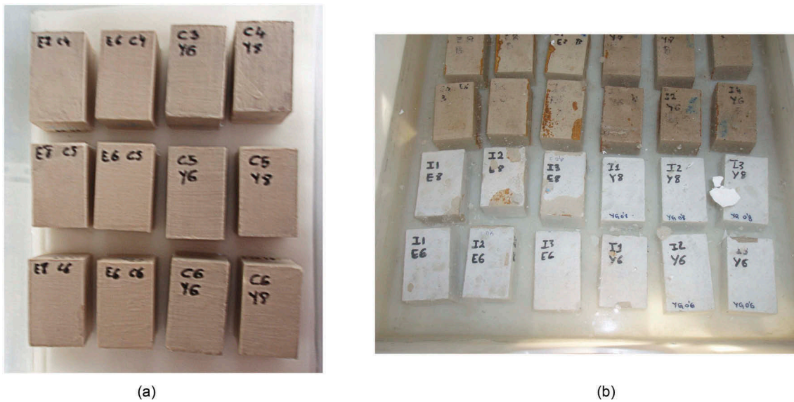
Figure 3. Weathering tests: a) Capillary water absorption, b) Absorption by immersion.
