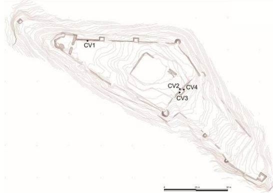
Fig. 4. Location of samples taken from defence walls and tower wall.
