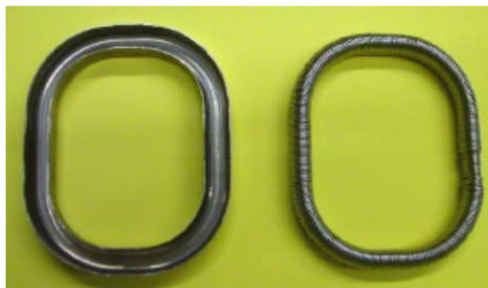
Figure 2.9 Rogowski coils used in JET with their protective case, reprinted from [22]
