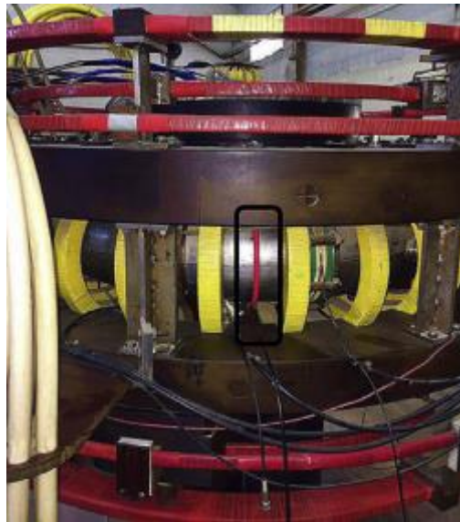
Figure 2.6 Rogowski Coil installed inside the Alvand Tokamak, reprinted from [17]
