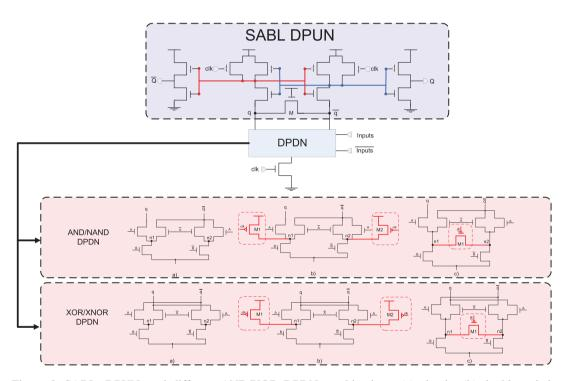
Figure 9. SABL, DPUN, and different AND/XOR DPDN combinations: (a) classic, (b) double-switch solution, and (c) single-switch solution. [Colour figure can be viewed at wileyonlinelibrary.com]
