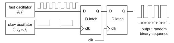
Figure 13. A schematic representation of the core structure of a TRNG exploiting high-jitter oscillators.
