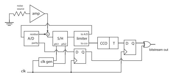
Figure 18. A TRNG exploiting a mixture of the three sources of randomness mentioned in Section 6: electronic noise, chaos, and oscillators sampling [93]. The A/D block, with analog residuals, is actually used to implement the Sawtooth chaotic map of Figure 11.
