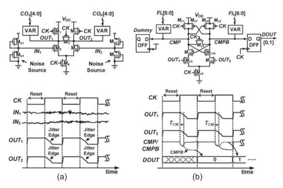
Figure 17. A TRNG exploiting electronic noise and metastability, generating one random bit DOUT each clock period (phase (a) and phase (b)) [145]. The VAR blocks are digitally controlled networks of varactors, to finely adjust the statistical biasing of the generated random sequences.
