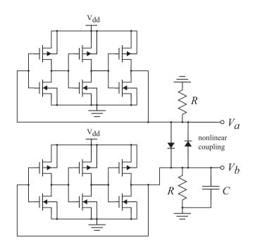
Figure 14. A nonlinear network coupling two ring oscillators have been proposed in [94] to implement a chaotic 'oscillator', to substitute the conventional fast oscillator in Figure 13.
