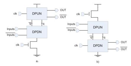
Figure 8. Dynamic and dual-rail gate logic style. (a) Using NMOS transistors to implement the DPDN block logic function. (b) Logic function implemented with PMOS transistors (DPUN). [Colour figure can be viewed at wileyonlinelibrary.com]
