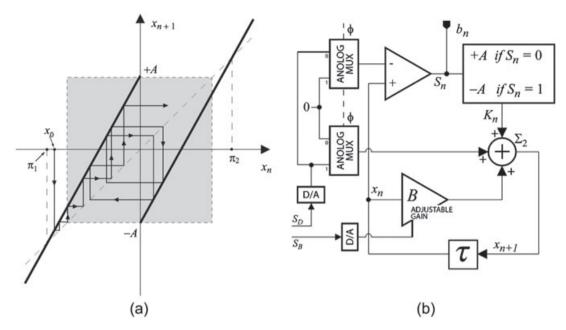
Figure 11. The Sawtooth discrete-time one-dimension piecewise linear map (a), and a TRNG exploiting this map with control signals to finely adjust the chaotic system parameters (b) [97]. In (a), the chaotic trajectory triggered by the initial condition  $x_0$  is shown using a cobweb plot [98]. The true random binary sequence is collected at the net  $b_n$  in (b).
