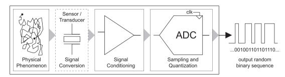
Figure 16. Schematic representation of the core structure of a TRNG exploiting the measurement of a stochastic physical process. When the stochastic source itself issues electric signals, as in the case of TRNGs based on electronic noise, the sensor/transducer is not necessary.
