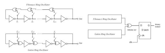
Figure 15. A TRNG exploiting Fibonacci and Galois ring oscillators [141].
