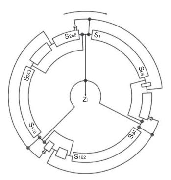
Figure 4. Simplified implementation of Trivium algorithm [9].
