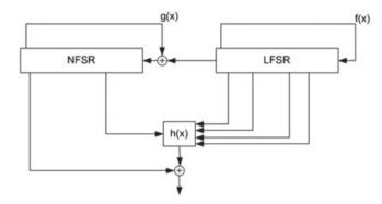
Figure 3. Simplified implementation of Grain algorithm [8].
