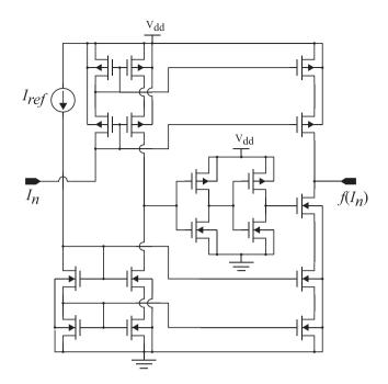
Figure 12. CMOS circuit to implement the algebraic calculation of the Sawtooth nonlinear function shown in Figure 11(a), using cascode current mirrors [111]. The chaotic state variable is represented by the current  $I_n$ .
