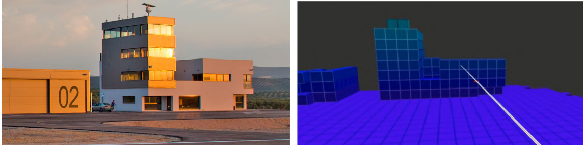
Figure 6.23: Left, ATLAS control tower. Right, RViz visualization of the octomap representation based on the LIDAR point cloud, and the conflictive flight plan under the ROS framework.
