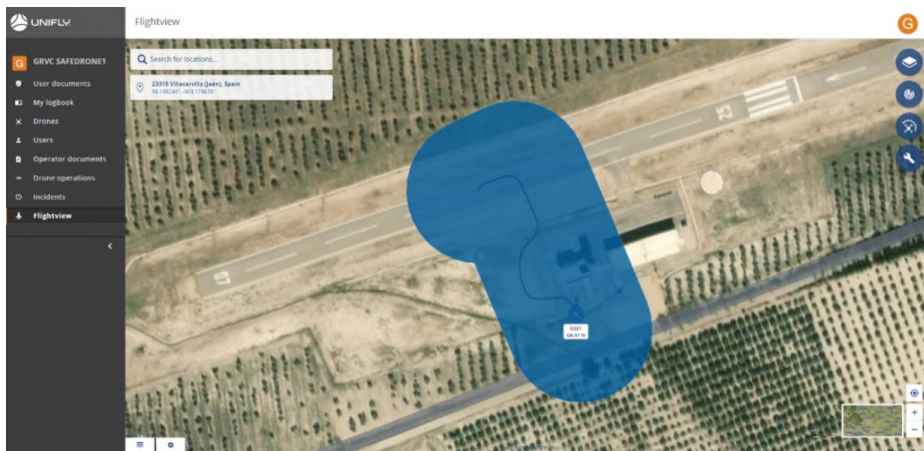
Figure 6.24: The Unify U-space Service Provider interface. Representation of the alternative flight plan carried out by the UAS and the OV reserved in the U-space system.
