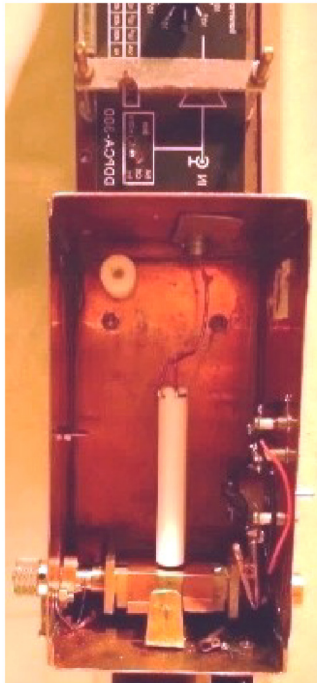
FIG. 1. The arrangement for supporting a sample by suspension to avoid degradation of transmitted current through supporting struts. The air in the FB is ventilated to minimize ions coupling charge to the sample.
