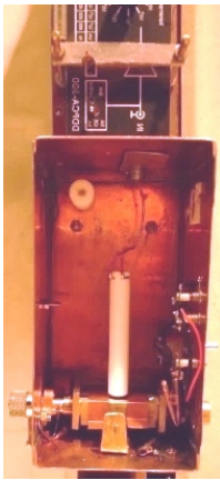
FIG. 1. The arrangement for supporting a sample by suspension to avoid degradation of transmitted current through supporting struts. The air in the FB is ventilated to minimize ions coupling charge to the sample.
