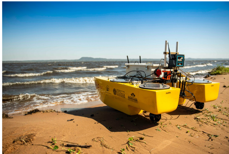
Fig. 1. ASV prototype for the monitorization of lake Ypacaraí (Paraguay). The ASV is equipped with water quality sensor modules, GPS and communications for remote planning.
