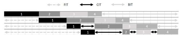
Fig. 1. Idle times in the PFSP: FIT front idle time; CIT: core idle time; BIT: back idle time
