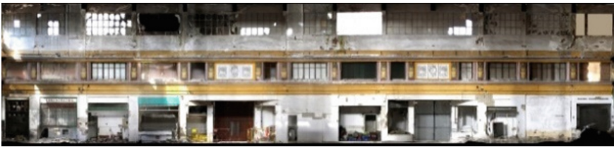
Fig. 6. Preliminary photogrammetric capture. Orthophoto of the interior façade. Author: Antonio Almagro Gorbea (2015).
