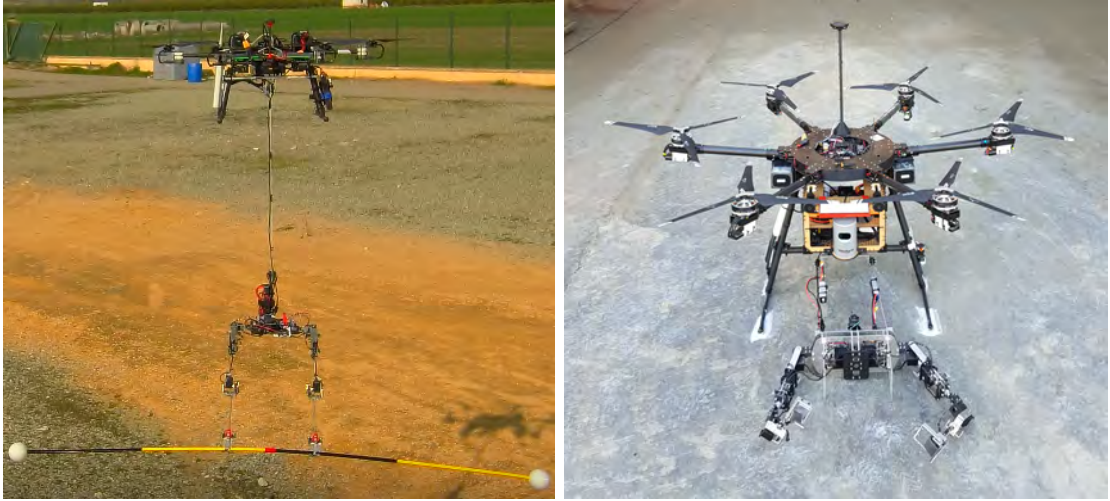
Figure A.8: Second version of a set of Aerial Robotic Systems for Long-Reach Manipulation (ARS-LRM_v2). First (left) and final (right) prototypes.
