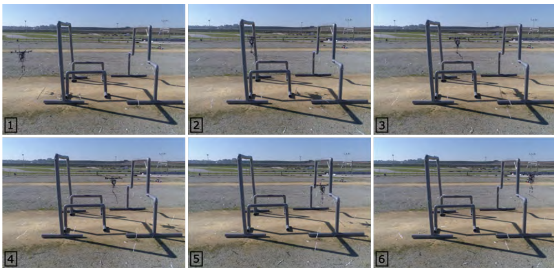
Figure 3.19: Long-bar transportation with in-flight planning capabilities. Snapshots of the operation.
