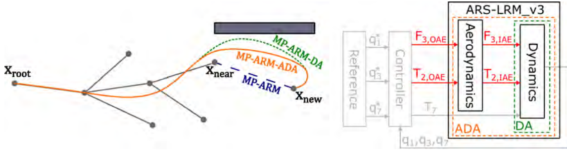
Figure 4.25: Operation basis of the MP-ARM-ADA algorithm (left) and closed-loop scheme required to perform the simulations that give support to it (right). The terms highlighted in red correspond to the variables employed to model the Aerodynamics Awareness.
