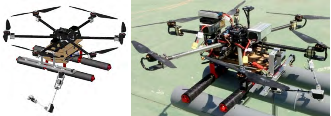
Figure A.15: Hybrid robotic manipulator (HRM) with aerial-rolling locomotion capabilities.
