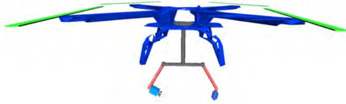
Figure A.1: First version of a set of Aerial Robotic Systems for Long-Reach Manipulation (ARS-LRM_v1).
