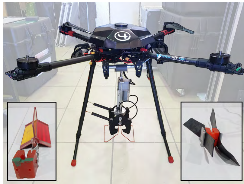
Figure A.18: Aerial Robotic Manipulator with Linear Actuator (ARM-LA) for the installation on power lines of clip-type bird diverters (bottom corners).
