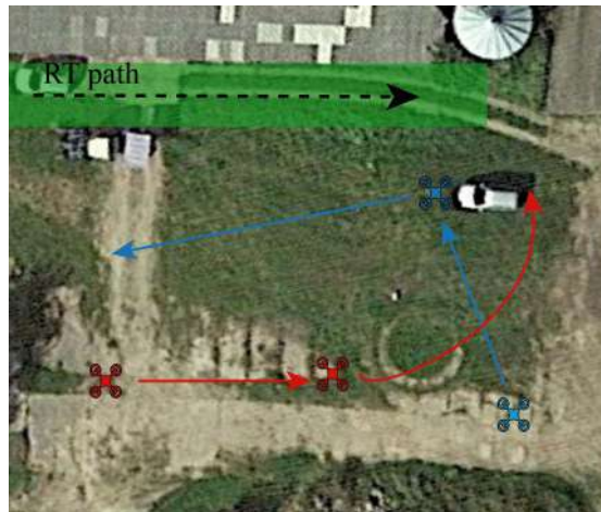
(a) Top view of the scene with the virtual target and the UAV trajectories for each Shooting Action. In green, the parkour area.
