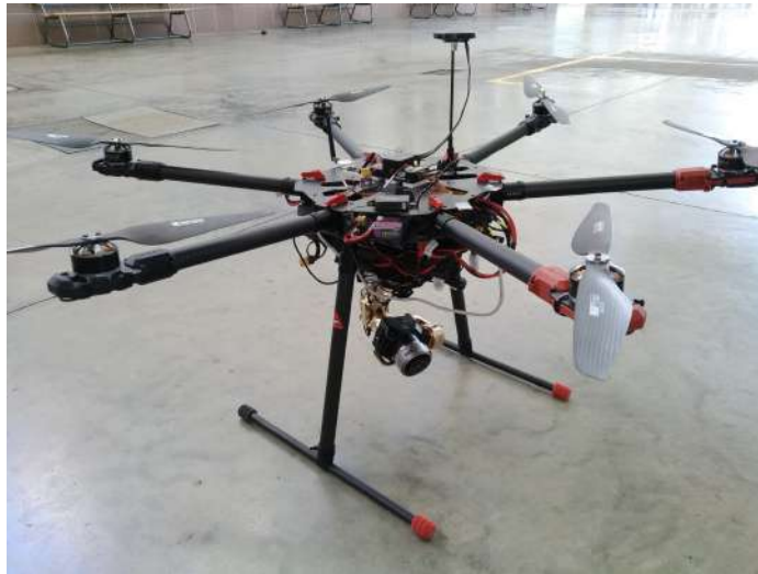
Figure 3.6: One of the UAVs used during our field experiments, with the cinematographic camera mounted on the gimbal.
