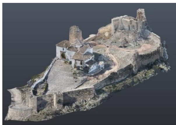
Figure 10: 3D model of the castle with the point cloud and mapping of high-resolution photos.
