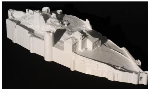
Figure 14: Initial 3D model of the castle of Carcabuey printed in high-resolution for the study of pathologies.
