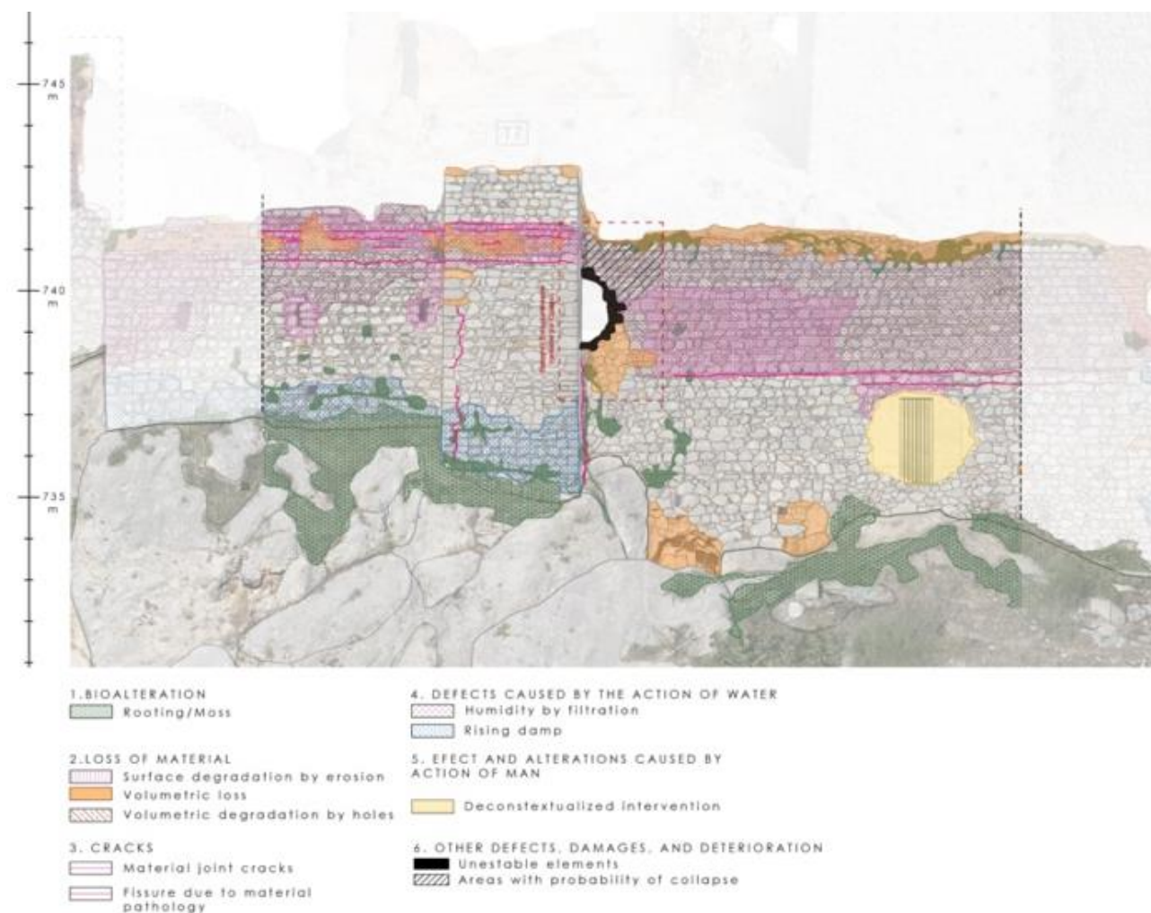
Figure 21: Study of material pathologies of the detail fragment of the wall studied from the model printed in high-resolution by the stereotomy of the construction.
