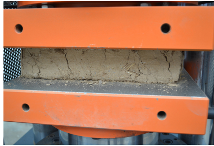
Figure 3: Failure mode of a brick tested in horizontal position.
