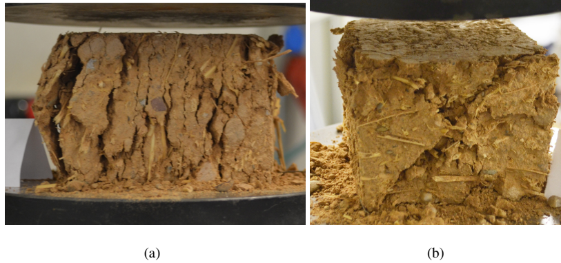
Figure 8: Typical mode of failure of (a) cubes loaded in transversal ( T ) direction (b) cubes loaded in longitudinal ( L ) direction (c) prisms and (d) cylinders
