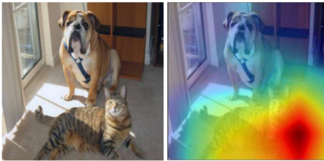
Fig. 5. Grad-CAM algorithm output example: class-discriminative regions of class 'Cat'. Images taken from Selvaraju et al. [32].
