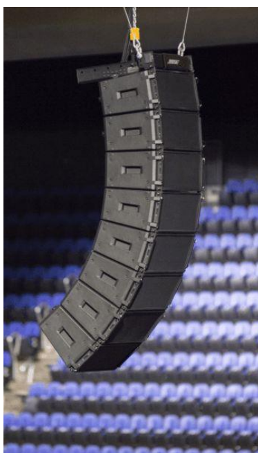
Figura 2.5 Line array Bose volado [11].
