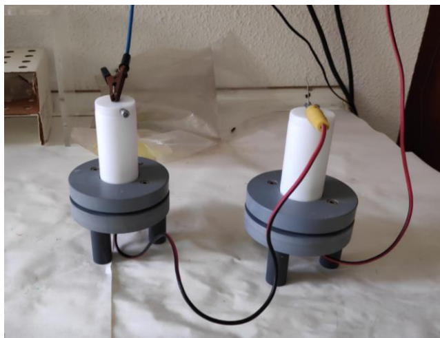
Figure 3.18: Electrodeposition set-up of two Pu samples in series
