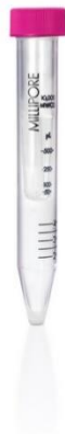
Figure 3.3.- Vial with the 3kDa filters embedded. Amicon Ultra-4 Centrifugal Filter Unit with Ultracel-3 membrane. We use this filter to separate between >3 kDa and <3kDa species.
