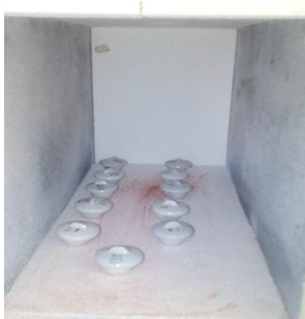
Figure 3.10.- Samples introduced at the muffle furnace (step 1n)
