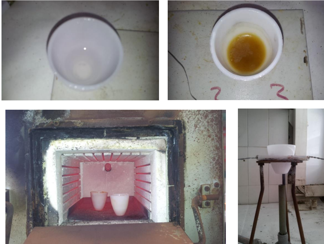
Figure 3.16.- Details of Alkali fusion. Left up is shown the melted salt dissolve impurities. Right up we show a sample properly dissolved. Down we can see the muffle furnace and the Bunsen burner, the two devices used to heat the samples.
