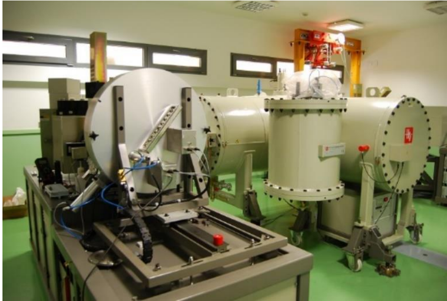
Figure 3.20.- S.A.R.A. Device for mass spectrometry techniques with accelerators.
