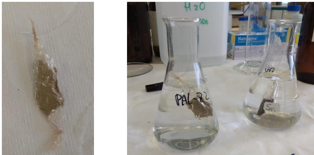
Figure 3.8.- Dialysis container filled with soil (left), and process of interaction container-physiological solution during the leaching experiment.
