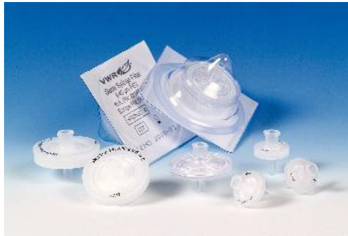
Figure 3.2.-. Syringe filters with Acrylic Housing 25 mm. Polyethersulfone with a pore size of 0.45 \mu m. Used to obtain the <0.45 \mu m size aliquots.
