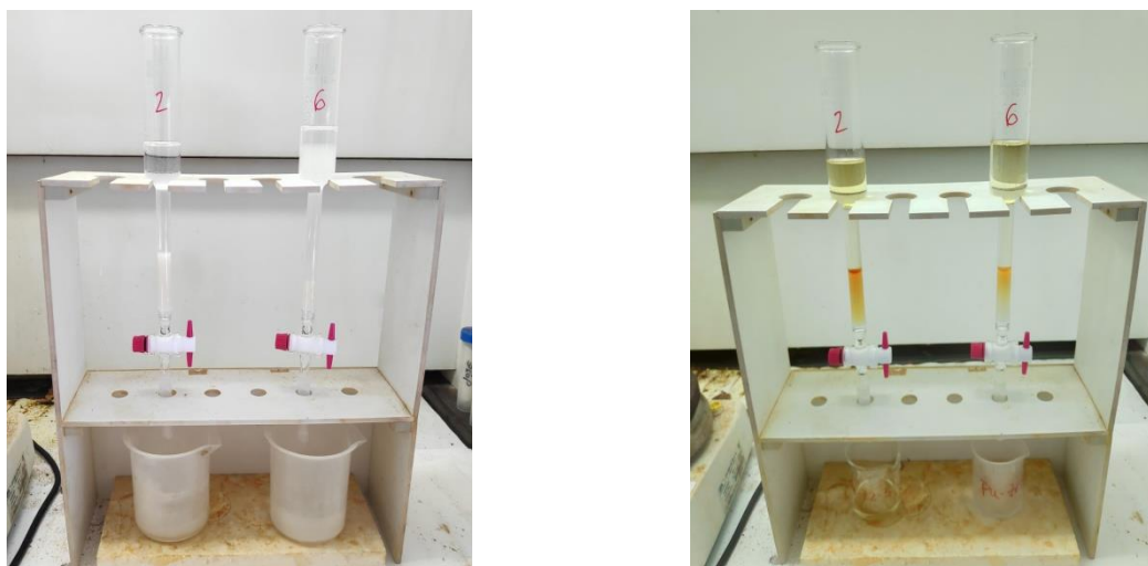
Figure 3.17.- a) Process of formation of the ion-exchange column (left), b) Process of stripping of Pu with the 1M \text{NH}_4\text{I}/9\text{M} HCl solution.
