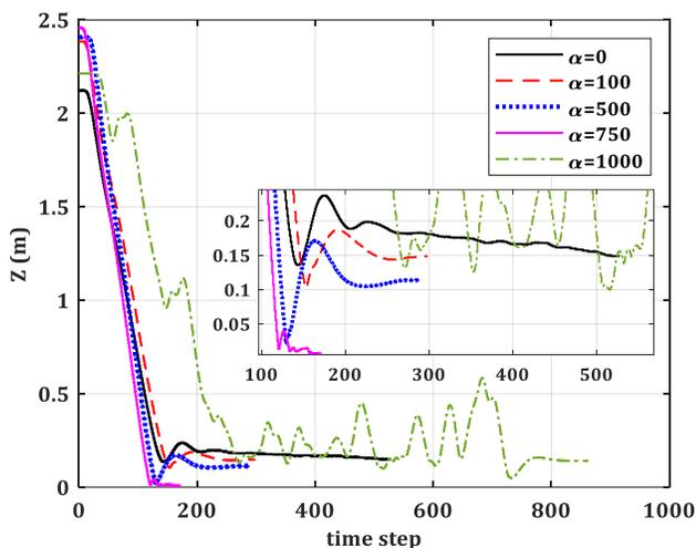
Fig. 4. The results of the soft-landing in  $Z$  axis direction with different selection of  $\alpha$ .
