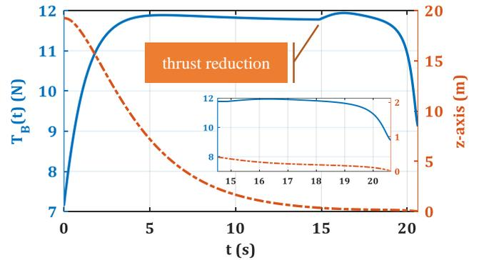
Fig. 3. Thrust reduction during soft-landing for a sample simulation due to feedforward thrust reduction.
