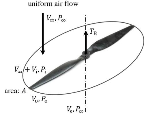
Fig. 1. Description of the momentum theory on a propeller.
