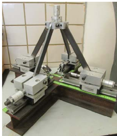
Figure 1. Device employed for biaxial tests.
