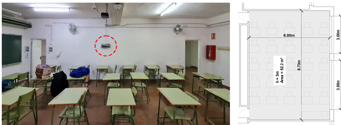
Figure 3. Typical distribution of analyzed classrooms. Placement of sensors.
