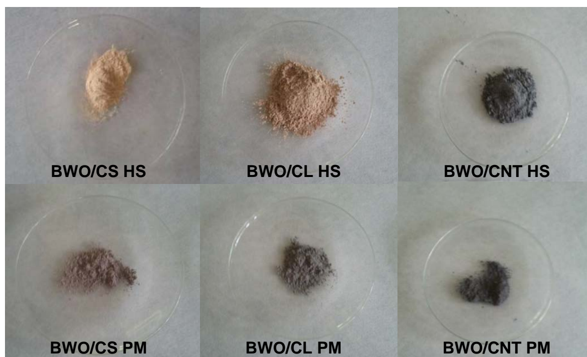
Figure 1. Images of hybrid catalysts prepared by incorporation of the carbon additive before the hydrothermal synthesis of the semiconductor (series HS) or by physical mixture of the carbon and \text{Bi}_2\text{WO}_6 powders (series PM).
