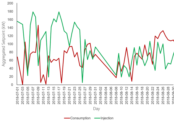
Figure 6.1 Aggregated Power Injection profile (green) vs Aggregated Power Consumption profile per day (red).
