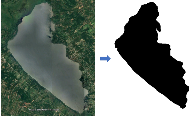
Figure 3.2 Example of a map model. Originally, the real image is drawn from a Satellite Resource. Then, it is translated to a binary image according to the navigability inside a square of a defined side d .
