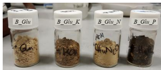
Figure 13. Samples of impregnated boehmite after drying at 100 \text{ }^\circ\text{C} for 16 h.
