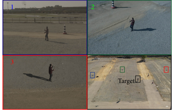
Figure 11: Example images from the cameras on board the UAVs during the experiment: top left, UAV 1 (blue); top right, UAV 2 (green); and bottom left, UAV 3 (red). Bottom right, a general view of the experiment with the three UAVs and the target.
