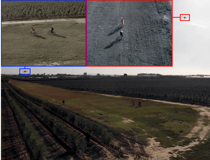
Figure 1: Cinematography application with two UAVs filming a cycling event. Bottom, aerial view of the experiment with two moving cyclists. Top, images taken from the cameras on board each UAV.
