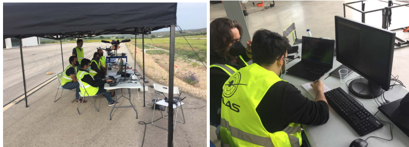
FIGURE 9. Setup for the experiments. On top, an view of the interfaces between the components run on each computer. The computers running the RPS for the two UAS and the UTM system were communicated through the internet via the MQTT protocol. At the bottom, pictures of the UAS Ground Control Station (left) and the UTM computer (right).
