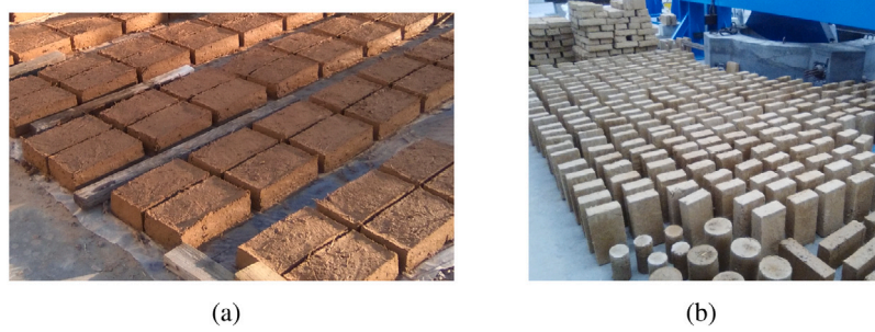
Fig. 1. Adobe bricks: (a) molded and air dried and (b) stored in laboratory conditions (temperature between 15 and 25 °C and humidity around 50%).
