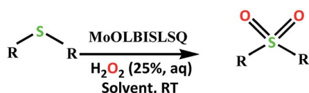
Scheme 7 Selective oxidation of sulfides to sulfoxides or sulfones catalyzed by MoOL BISL SQ.
