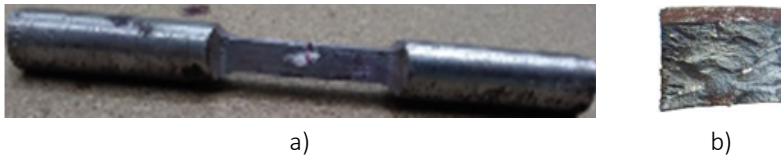
Figure 2. Tested specimens. a) Crack measurement (3,8 mm) in the specimen number 2. b) Specimen number 2 cross section failure.
