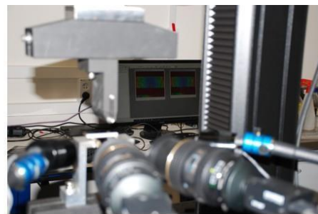
Three-point bending setup with DIC
