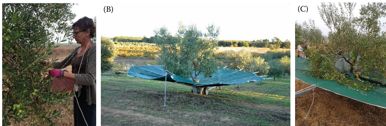
Figure 1. Harvesting methods: Manual harvesting using a macaco (A); and the manual inverted umbrella prototype (B) and a branch vibrator (C)
