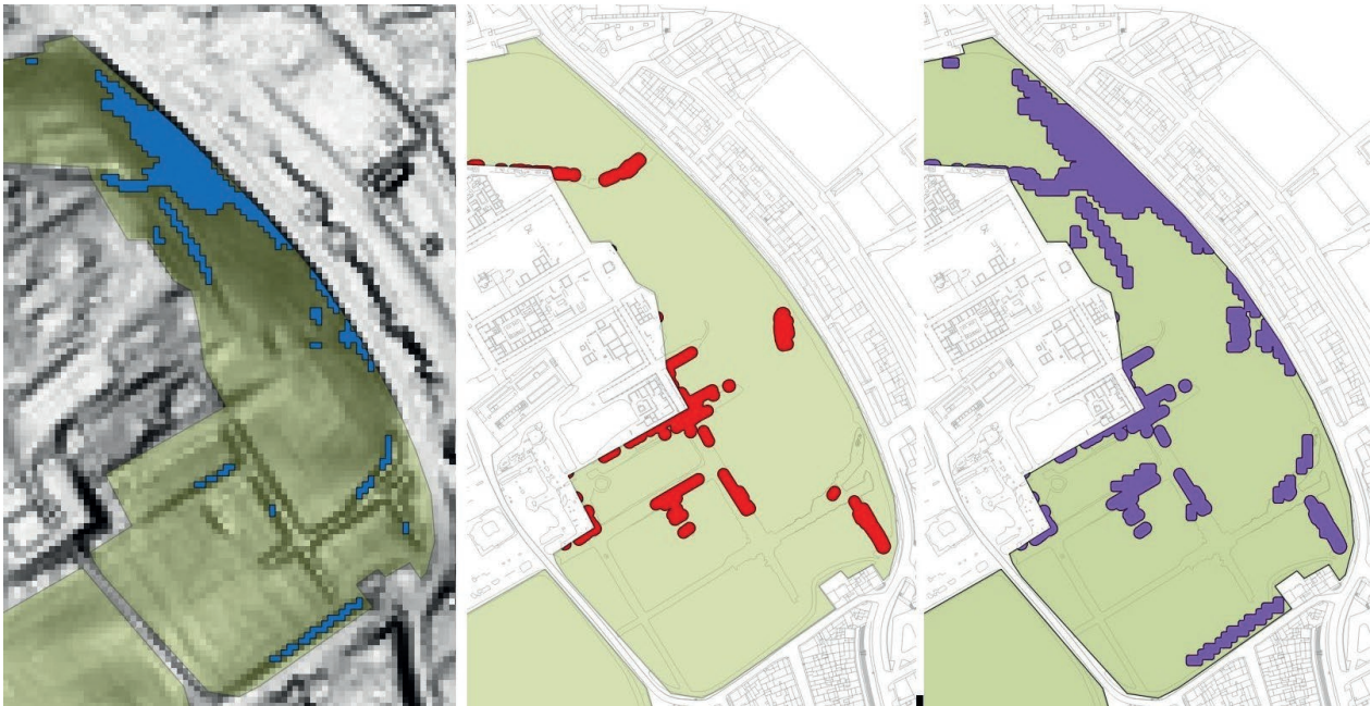
Fig.19. GIS analysis of vegetation clearance in the archaeological reserve areas: gradient of over 15% (blue), proximity to remains (red) and areas where the use of machinery is restricted (purple). (Source: The authors).
