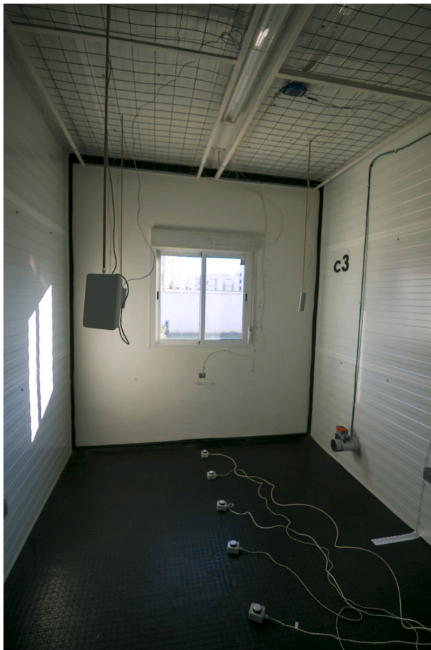
Fig. 5. Test cell used for the comparison trials. (A) Test cell with the array of illuminance-meters above the floor. (B) and (C) DA, DA con and DA o results obtained from simulation calculations and illuminance measurements for 250 and 500 lx.
